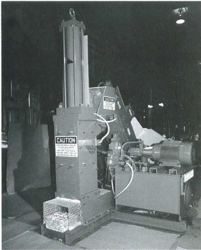
Rear view of PAK-A-CAN™ compression unit with multi-stroking ram. The compression chamber is fully protected by abrasion-resistant plates which are through-bolted for easy replacement. A bisquette under the mesh guard has been ejected from compression chamber.
